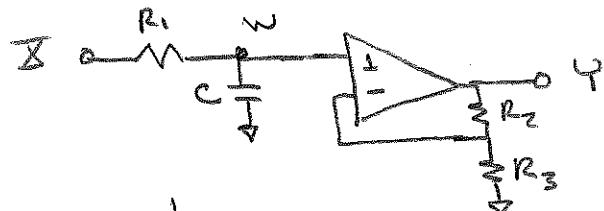
$$\frac{Y}{X} = \frac{\frac{1}{R_1 C}}{s + \frac{1}{R_1 C}} \quad \frac{Y}{X} = \frac{R_2 + R_3}{R_2}$$
