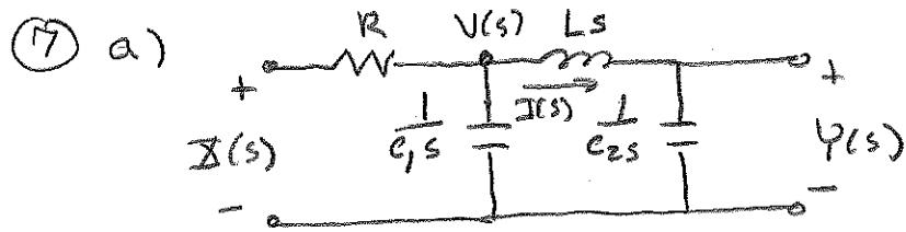
b) KCL at  $V(s)$ :  $\frac{I - v}{R} = C_1 s V + I \quad (1)$
