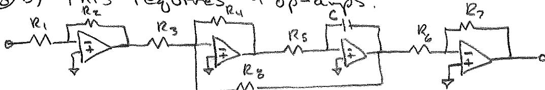
$$\text{where } k_0 = \frac{R_2}{R_1} \quad k_1 = \frac{R_4}{R_3} \quad k_2 = \frac{R_4}{R_5} \quad k_3 = \frac{1}{R_5 C}$$
