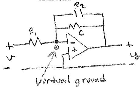
KCL at inverting input
