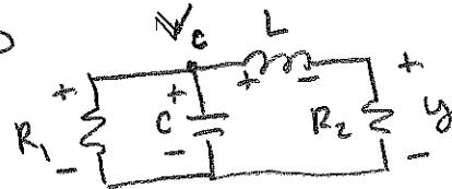
$$\textcircled{1} \text{ KCL at } V_c \quad \frac{V_c}{R_1} + C V_c' = i$$
