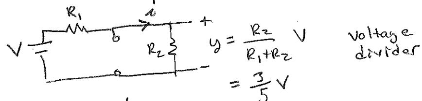
$$\text{so } y(0) = \frac{3}{5} V, \quad y = R_2 i \Rightarrow y' = R_2 i' \Rightarrow y'(0) = 0$$
