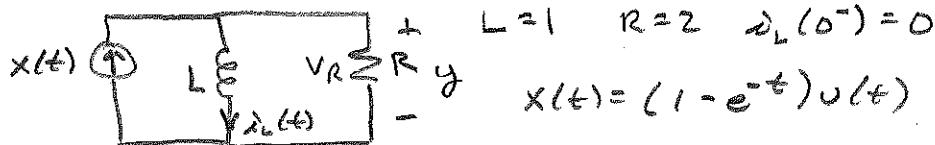
$$\text{KCL: } \omega_L + \frac{V_R}{R} = x \quad \text{and} \quad V_L = V_R = L\omega_L'$$
