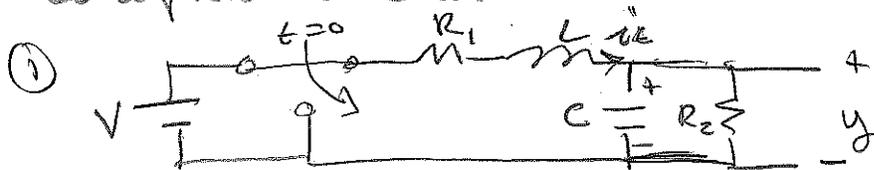
a) Determine the initial conditions on energy storage elements,  $i_L$  &  $V_C$ .
