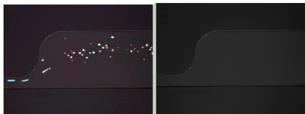
Figure 3: One, of 20 randomly selected, input frame used for calculating the background image using a median filter on left and resultant background image on right.
